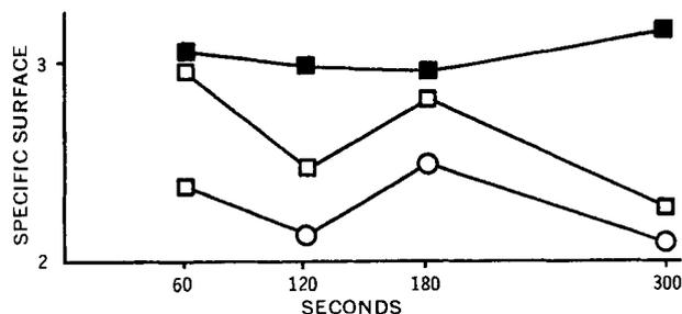
**Figure 6**—Specific surface values of mineral oil-in-water emulsions prepared with various HLB values at surfactant concentrations of 1.5% and a power level of 80. Key: ■, HLB 11.3; □, HLB 10; and ○, HLB 9.
