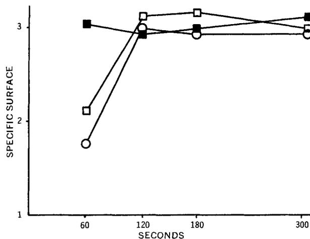
**Figure 7**—Specific surface values of mineral oil-in-water emulsions at various power levels and optimal surfactant (1.5%) and HLB (11.3) levels. Key: ■, power level 80; □, power level 65; and ○, power level 55.
