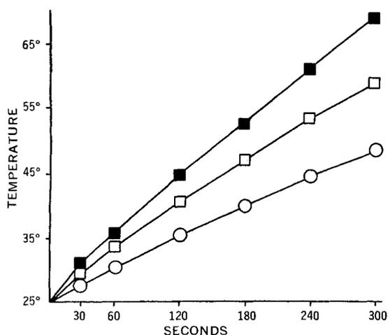
Figure 2—Determination of Sonifier power levels calorimetrically. Key: ■, power level 80; □, power level 65; and ○, power level 55.
