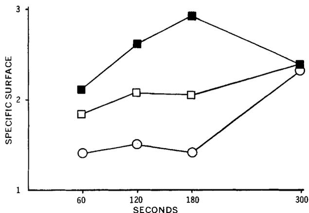
**Figure 4**—Specific surface values of mineral oil-in-water emulsions prepared at various ultrasonic power levels at surfactant concentrations of 1.0% and an HLB of 10. Key: ■, power level 80; □, power level 65; and ○, power level 55.
