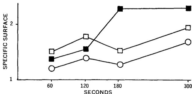
Figure 3—Specific surface values of mineral oil-in-water emulsions prepared at various ultrasonic power levels at surfactant concentrations of 0.5% and an HLB of 10. Key: ■, power level 80; □, power level 65; and ○, power level 55.
