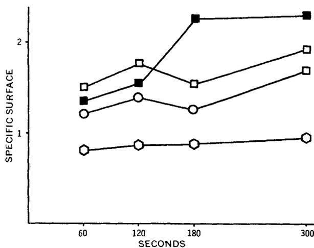
**Figure 8**—Comparison of specific surface values of mineral oil-in-water emulsions prepared ultrasonically and with a Homomixer at surfactant concentrations of 0.5% and an HLB of 10. Key: ■, power level 80; □, power level 65; ○, power level 55; and ○, Homomixer.
