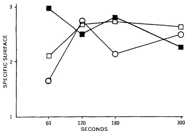
**Figure 5**—Specific surface values of mineral oil-in-water emulsions prepared at various ultrasonic power levels at surfactant concentrations of 1.5% and an HLB of 10. Key: ■, power level 80; □, power level 65; and ○, power level 55.
